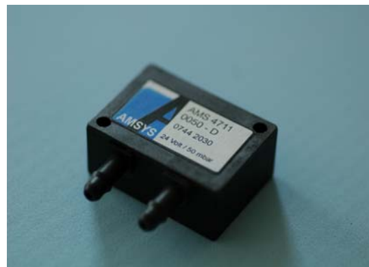
Figure 10: Pressure sensor in a plastic casing (transmitter), example: AMS 4712 [3]
