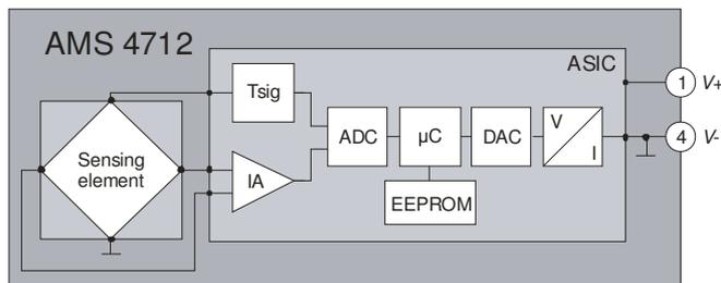
**Figure 3:** Block diagram of transmitter AMS 4712
