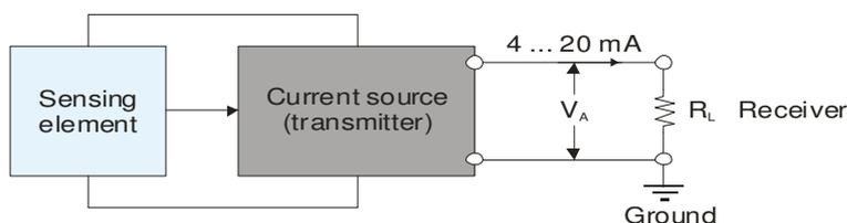
**Figure 2:** Schematic diagram of a sensor with a 4 – 20 mA output
