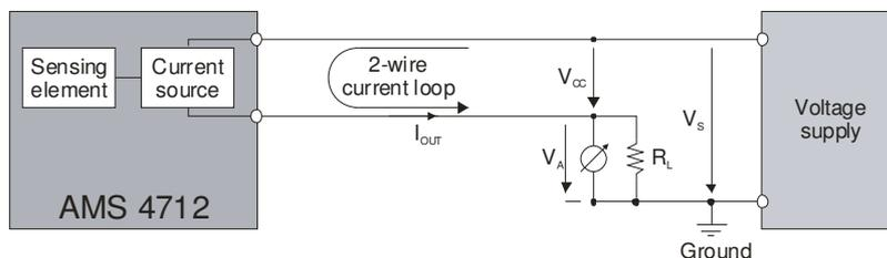
**Figure 4:** Practical application of the current loop circuit
